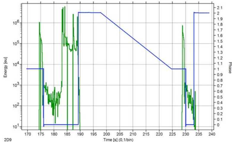
Fig. 6 Energy rate for a damaging (left) and a good crimping of an FRP rod.
