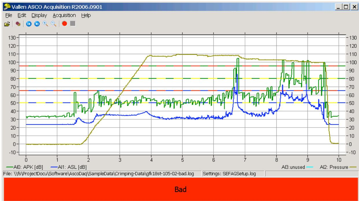
Fig. 10 A screen after a damaging crimping.
