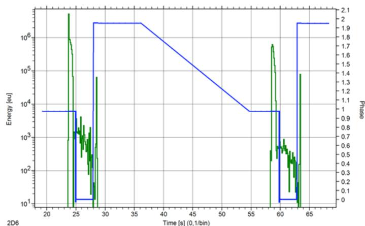
Fig. 5 Energy rate during steel-rod-crimping.
