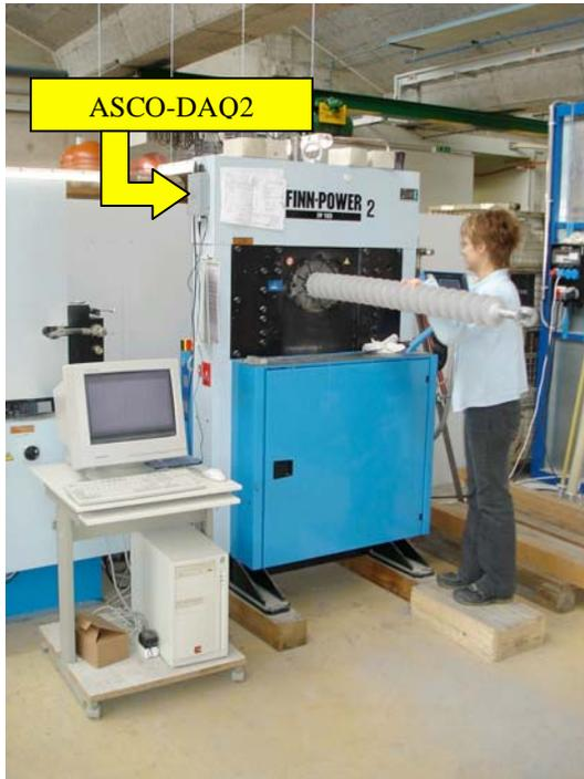
Fig. 7 ASCO-DAQ2 mounted to hydraulic press.
