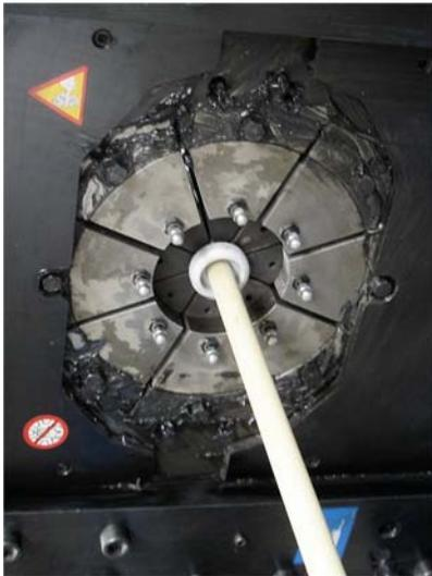
Fig. 1 Crimping an end-fitting onto a rod.
