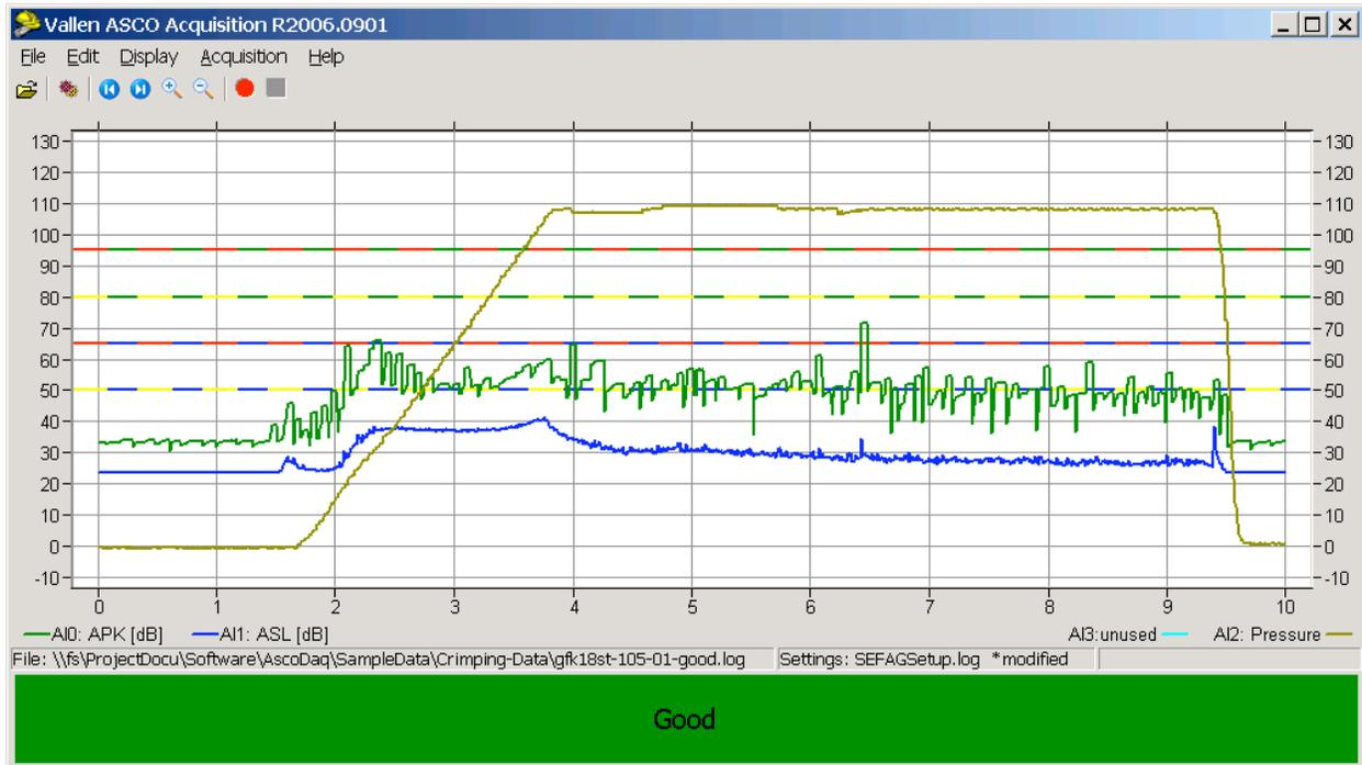
Fig. 9 An example for a good crimping screen.
