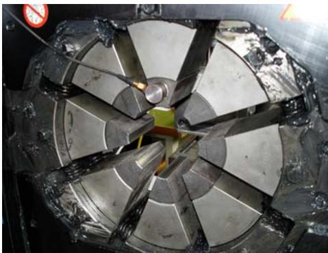
Fig. 4 Sensor bonded to the fixed crimping claw.
