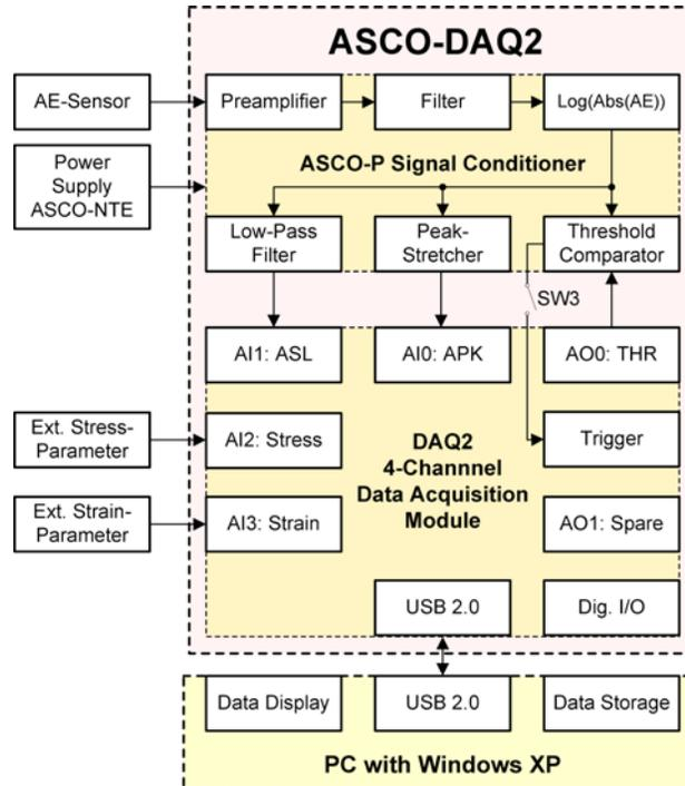
Fig. 8 ASCO-DAQ2 hardware schematic.
