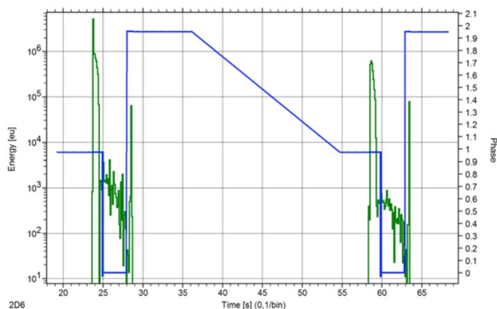
Fig. 5 Energy rate during steel-rod-crimping.
