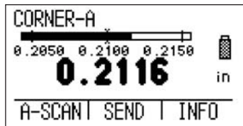
Numerical value of thickness is filled when probe is coupled to the location of measurement
