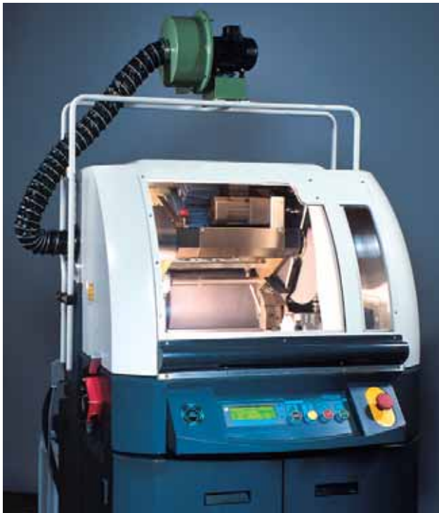
The 10-2342 Fume Extractor filters and reduces emissions.
