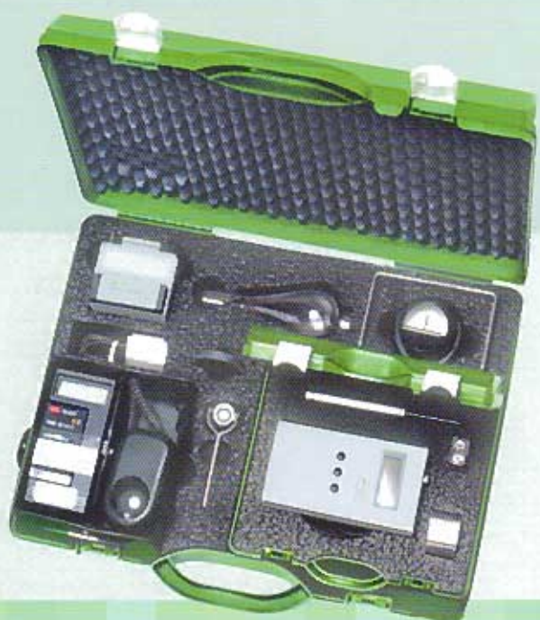
Measuring instruments and test pieces for a successful and reproduceable magnetic particle inspection
