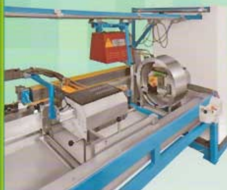
Special test bench to check parts for the aircraft and aerospace industry in accordance with all national and in- ternational standards. Yoke magnetization, coil magnetization and
