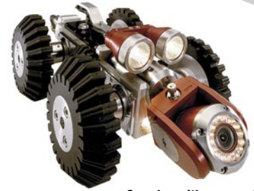
Crawler with pan-and-tilt camera and auxiliary lights on top
