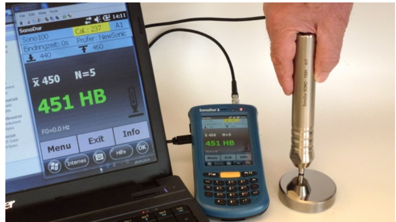
Fast and precise hardness tester SonoDur2 on GGG 50 cast iron and remote control via PC
