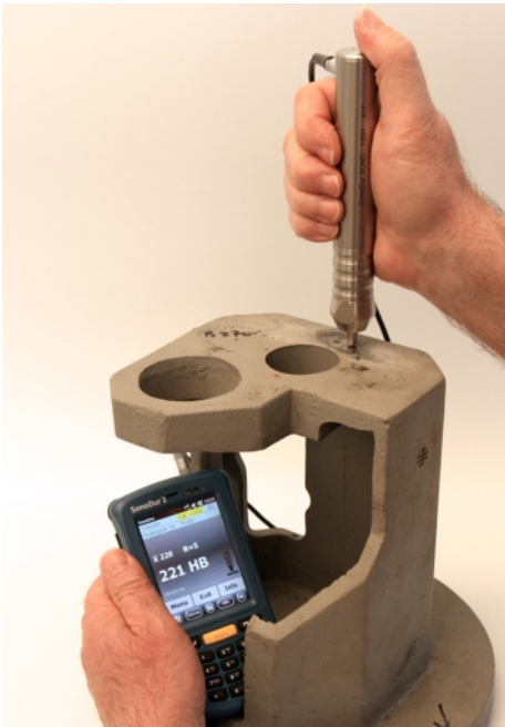
Fast and precise hardness tester SonoDur2 on GGG 50 cast iron and remote control via PC
