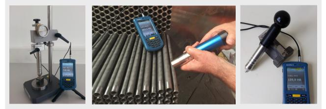
Testing of small parts using the modular, mobile test stand SONO-PS1 (left). SONO-S with selfcentering feature - the mobile test stand for perfect results on tubes, bars, rolls, profiles etc. (middle). SONO-100H HV 10 (10 kgf) probe with ball head (right), fatigue-free testing especially with high loads.
