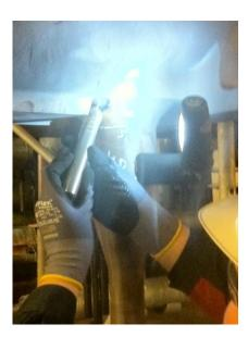
Prerequisite for a steady hardness test: Surface must be clean and smooth according to spec. (DIN 50159-1). In addition the procedures described in the standards need to be considered (DIN 50159, ASTM A 1038).
