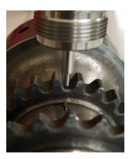
SONO-10H, HV 1 (10 N): Weld seams (HAZ), soft spots, nitrided & hard surface
