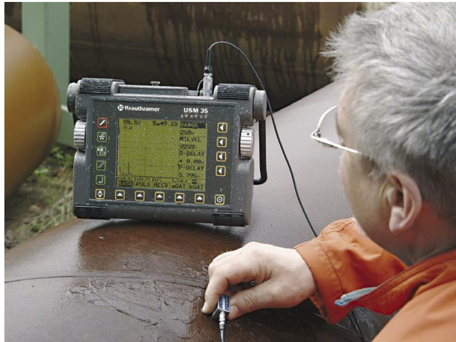
Inspection of a weld
