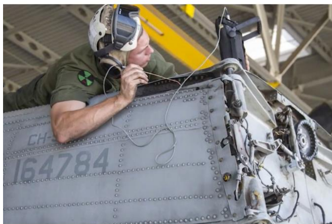
Crack Detection Around Fasteners
